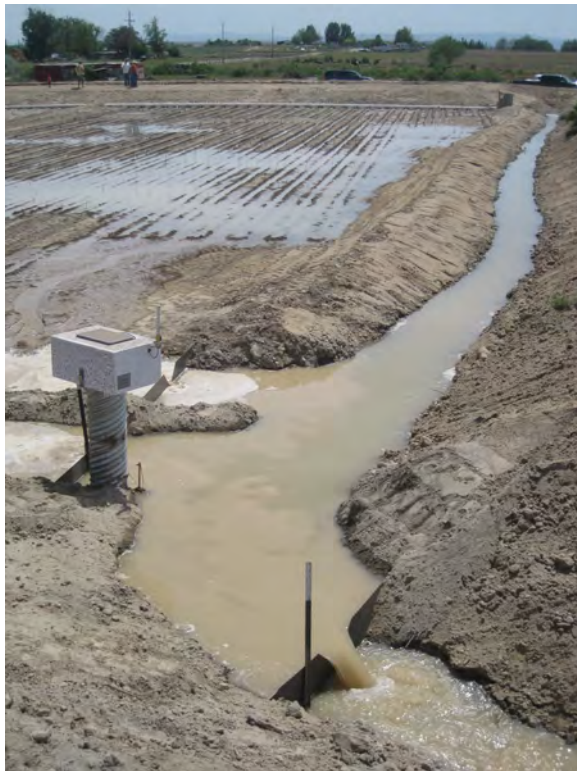
Figures 8A and 8B - Bypass Ditch, Flow Measurement Device, and Calibrated Weir
