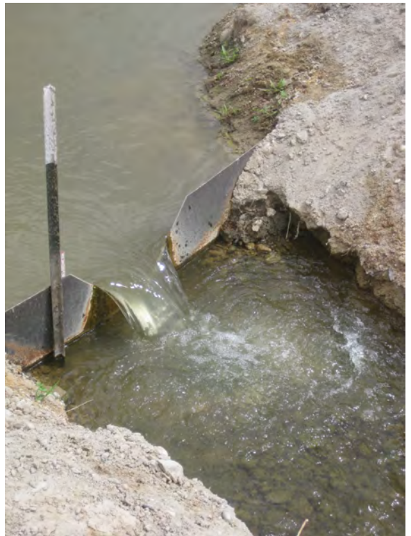
Figures 8A and 8B - Bypass Ditch, Flow Measurement Device, and Calibrated Weir
